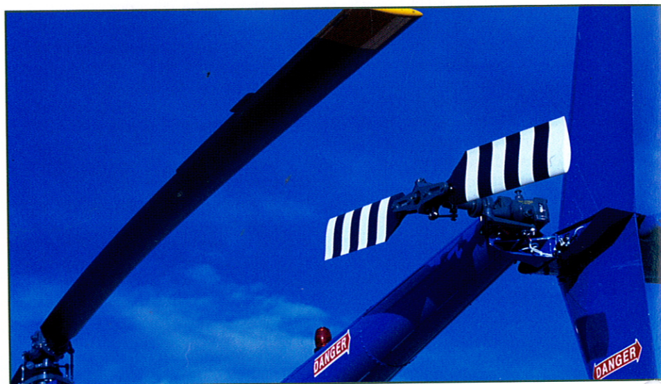
The Raven II's IO-540 fuel-injected piston engine, top, produces 300 hp. Robinson derated the engine to 245 hp for takeoff and 205 hp for continuous operation to extend the life of the engine. The tail-rotor blades, bottom, are attached to a teetering hub with a fixed coning angle.
