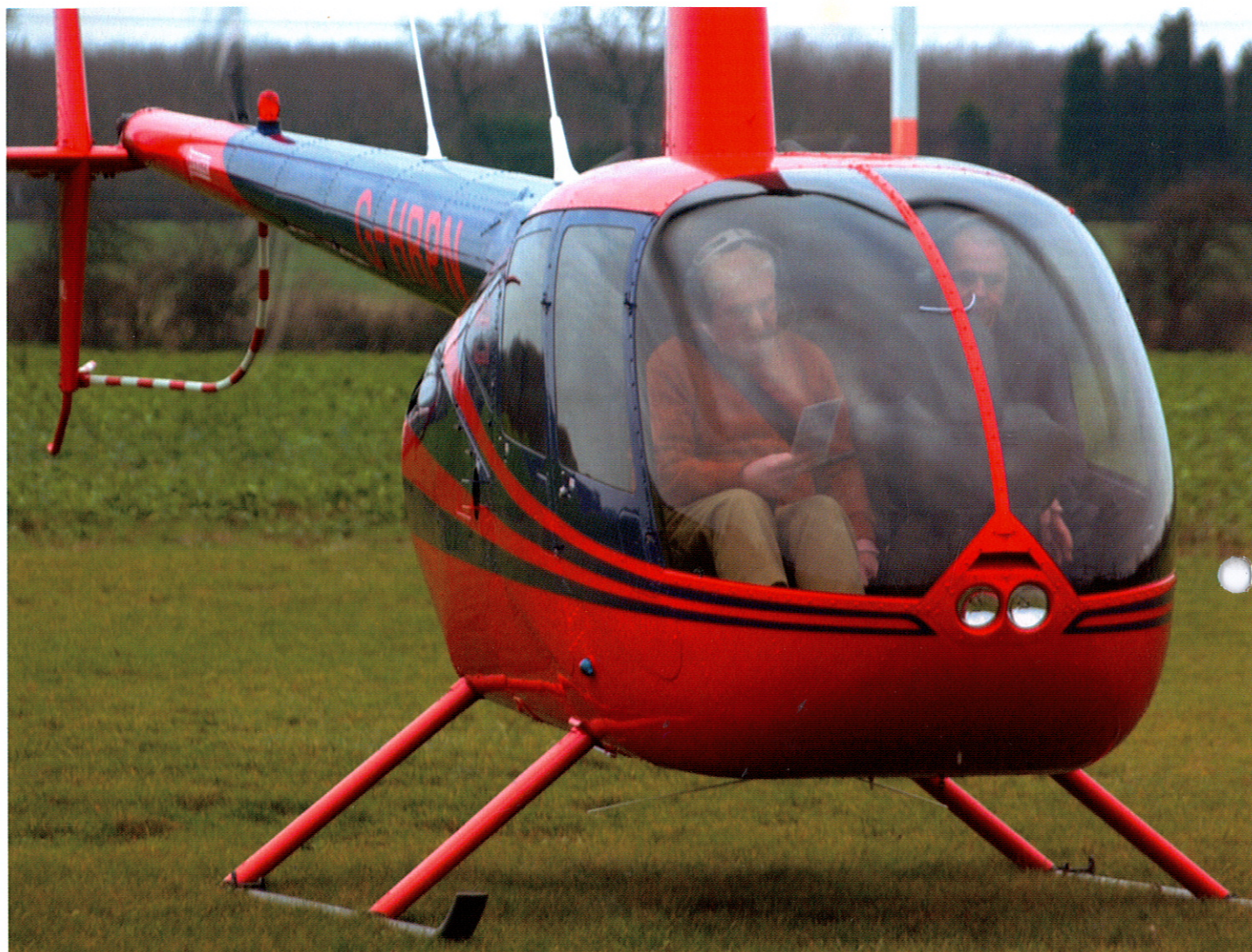
Above: Mike Green, right seat, runs through the shutdown procedure—switch off the governor, reduce power to 70 per cent, wait for CHT to drop, throttle closed, clutch out, pause 30 seconds and pull the mixture out.
